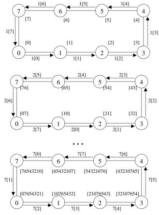
For the **ring** topology each processor can initiate sending its message simultaneously (in any chosen direction in the ring). At any moment of time each processor receives and sends data. The multinode broadcast operation will be terminated in (p-1) data communication steps.
