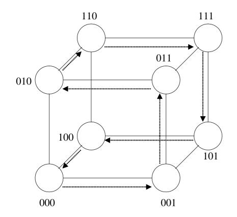
The essential characteristic of the Gray code is the fact that the neighboring values G(i,N) and G(i+1,N) differ only in a bit position. As a result, the neighboring nodes in the ring topology are mapped onto the neighboring hypercube processors.
