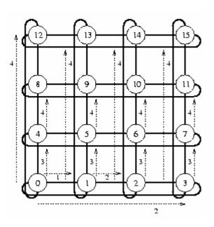
For the **grid-torus topology** broadcasting can be carried out as a two-stage procedure. At *the first stage* data are transmitted to all the processors of the network, which are located on the same horizontal line of the grid as the sending processor. During *the second stage* the processors, which received the data copy at the first stage, send the messages along the corresponding vertical lines.
