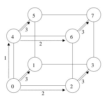
For the **hypercube** broadcasting can be carried out as an N-stage data communication procedure. During *the first stage* the sending processor sends data to one of the neighbors. As a result, there are two processors, which have the copies of the data after the first stage. At *the second stage* the two processors engaged at the first stage send messages to their neighbors along the second dimension, etc.
